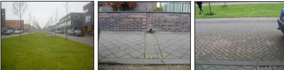
*Fig. 4. Wadi between roads and tiled pervious surfaces. Roof runoff is led onto the street to infiltrate or flow on the surface to the wadi.*
