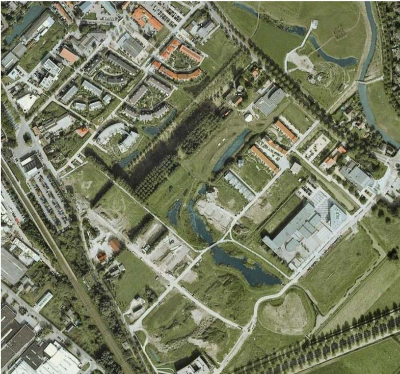
*Fig. 12. Orthographic photo showing EVA-Lanxmeer during construction. Note the lakes, the forest strip, the intimate gardens in top and the constructed wetland immediately next to the big building to the East. Elevation 1 km © Google Earth*
