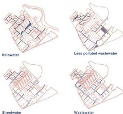
Fig. 11. Diagram of the 4 flows of wastewater at EVA-Lanxmeer
